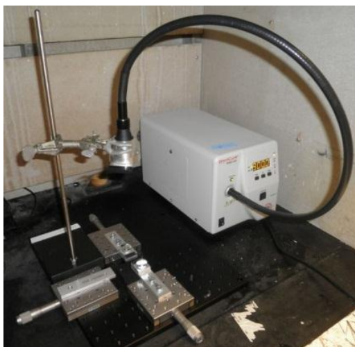
Figure 24. Experimental set up with the mercury arc lamp and uniaxial strain tester in the UV hood used in the curving and bending experiments
